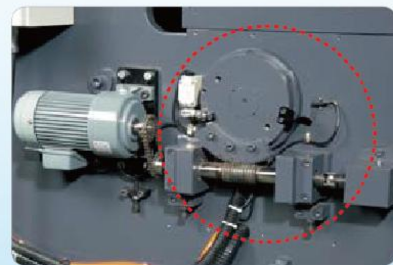
▲ 刀隙調整結構系統(蝸桿蝸輪) Blade Clearance Adjustment System (Wormgear)
