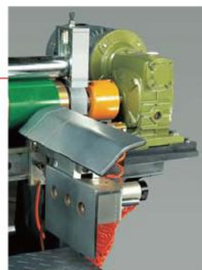
▲ 活動式左右側扶料機構 Movable right and left side stacking correcting flapper
